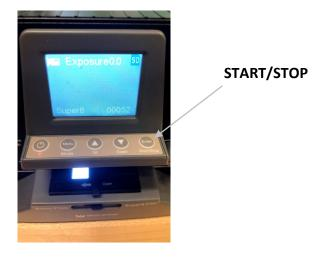
**2.** To stop recording, press the **STOP/START** button again. The scanner will now write the movie to the memory card into MPEG4 (MP4) digital movie files at 720p / 30 fps.
