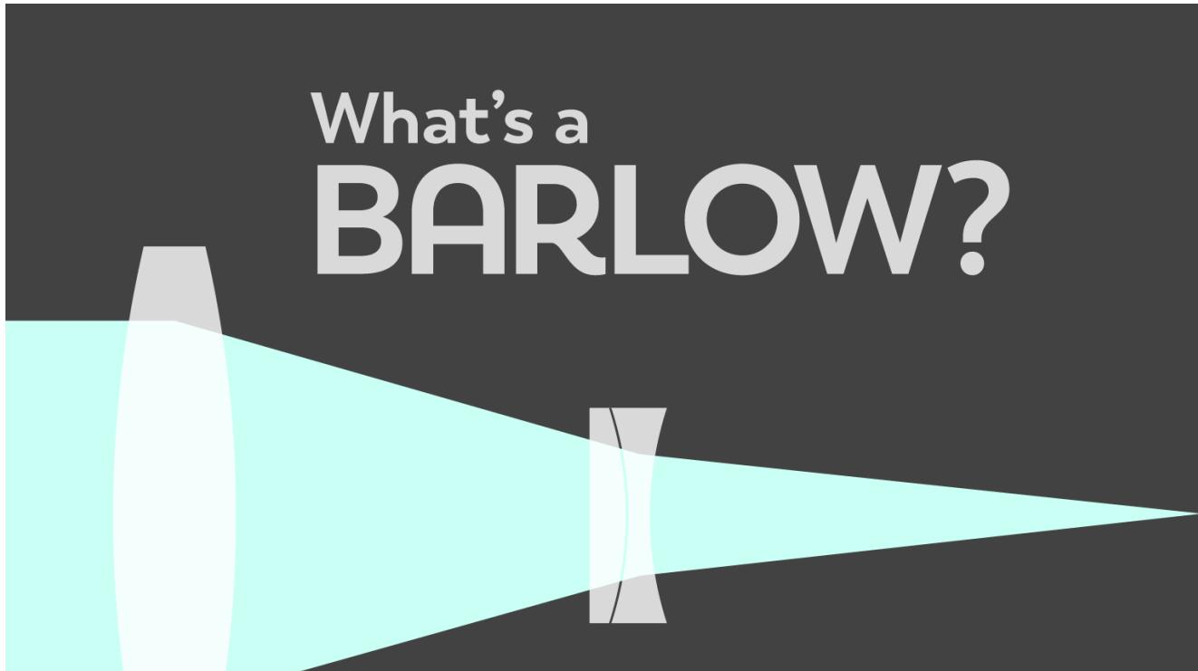
A Barlow lens is a type of lens that can **increase the magnification of your telescope**. The most common type is a **2x Barlow**, which doubles the magnification, but you can also find them in other magnifications, such as **3x** and **5x**.
