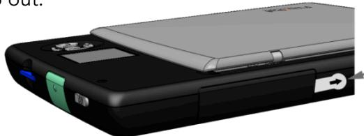
Press gently on battery door while pulling tab sideways to remove
